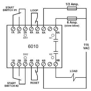
Be sure that electrical power is turned off before attempting to make wiring connections to the control. Make electrical connections according to the wiring diagram above. Use 18 gauge stranded copper wire that can withstand 60/75 degrees C. Tighten the wiring terminals to 1.0Nm. To protect the output contacts, a fuse (6A slow blow or 8A fast blow) should be connected before the output contacts as shown in the wiring diagram.
