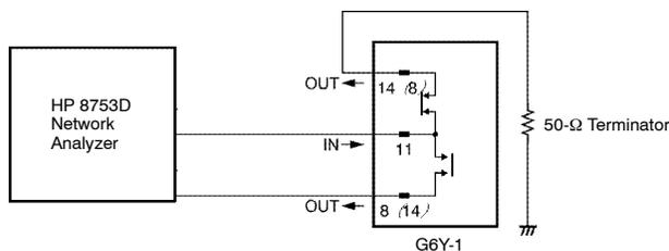
Terminals which were not being measured were terminated with 50  $\Omega$
