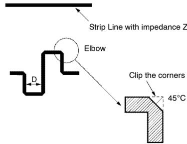
When the lines must curve, an elbow can be used as shown in the diagram. A distance (D) between the lines of approximately twice the line width is sufficient.
