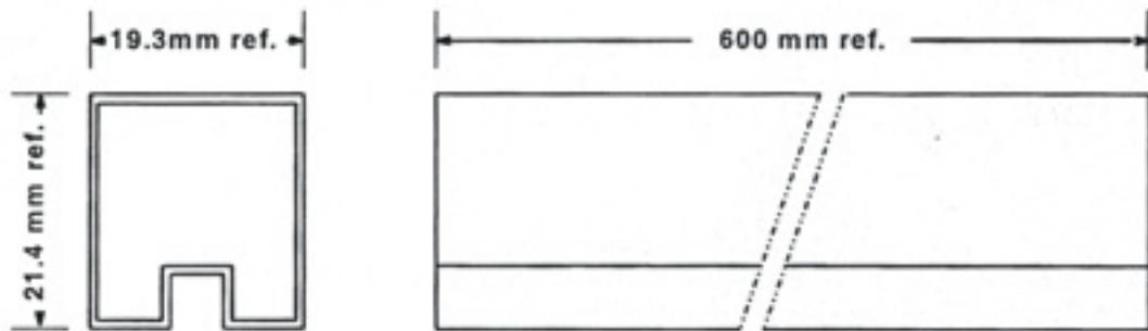
G8QN: 47 relays per tube, 36 tubes per box (1692 relays per box).
