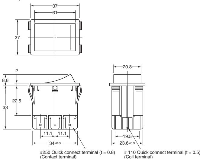
**Note:** Unless otherwise specified, a tolerance of  $\pm 0.8$  mm applies to all dimensions.
