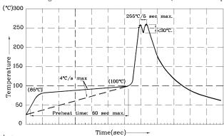
Notes: 1.Recommend pre-heat temperature of 105°C or less (as measured with a thermocouple attached to the LED pins) prior to immersion in the solder wave with a maximum solder bath temperature of 260°C 2.Peak wave soldering temperature between 245°C ~ 255°C for 3 sec
