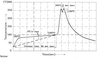
I.Recommend pre-heat temperature of 105°C or less (as measured with a thermocouple attached to the LED pins) prior to immersion in the solder wave with a maximum solder bath temperature of 260°C
