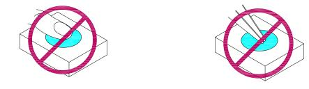
3. Do not stack together assembled PCBs containing exposed LEDs. Impact may scratch the silicone lens or damage the internal circuitry.
