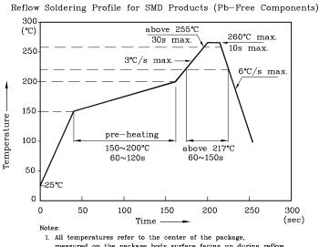
measured on the package body surface facing up during reflow. 2. Do not apply any stress to the LED during high temperature conditions. 3. Maximum number of soldering passes: 2
