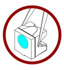
2. Do not directly touch or handle the silicone lens surface. It may damage the internal circuitry.
