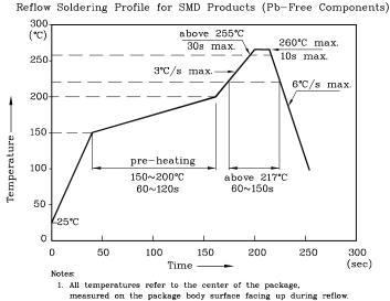
2. Do not apply any stress to the LED during high temperature conditions 3. Maximum number of soldering passes: 2
