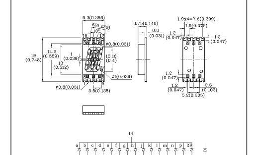
1. All dimensions are in millimeters (inches), Tolerance is ±0.25(0.01")unless otherwise noted.
