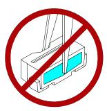
2. As silicone encapsulation is permeable to gases, some corrosive substances such as H<sub>2</sub>S might corrode silver plating of leadframe. Special care should be taken if an LED with silicone encapsulation is to be used near such substances.
