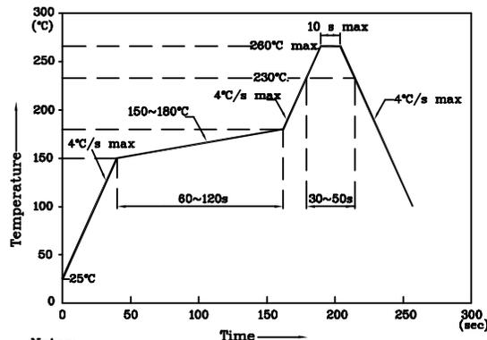
1. Maximum soldering temperature should not exceed 260°C
