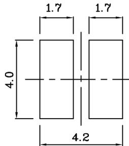
❖ The device has a single mounting surface. The device must be mounted according to the specifications.
