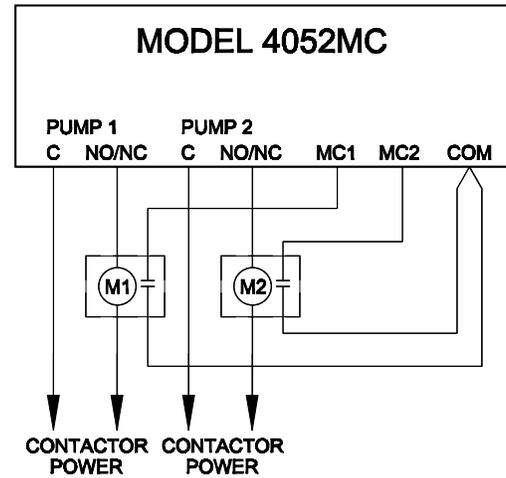
The 4052MC option replaces seal fail monitoring with motor starter monitoring. When the 4052MC calls for a pump to run the corresponding MC contact should close. If the MC contact closes, the pump controller will increment the run time for that pump. If the MC contact does not close, or opens after the pump has been started, the pump controller will not increment the run time for that motor and will flash the Run Time light on the left side of the controller for the corresponding pump.
