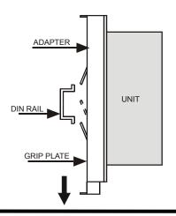
Once the unit is attached to the Adapter, place them both in position next to the 35mm DIN rail. Pull down on the movable part of the grip plate, and position the Adapter (with mounted unit) onto the DIN rail.
