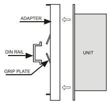
Note: for a better grip of the unit to the adapter plate, Locktite (Blue Dot) is recommended.
