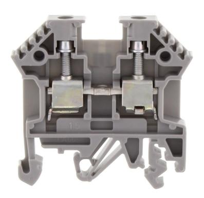
Feed-through terminal, Screw connection, Mounting type:Mounting rail TS 35/7.5 and TS 32, Rated cross-section: 4 mm², Width: 6 mm, Colour: Grey
