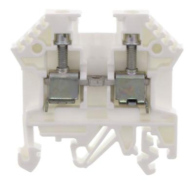
Feed-through terminal, Screw connection, Mounting type:Mounting rail TS 35/7.5 and TS 32, Rated cross-section: 4 mm<sup>2</sup>, Width: 6 mm, Colour: White
