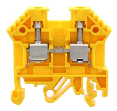
Feed-through terminal, Screw connection, Mounting type:Mounting rail TS 35/7.5 and TS 32, Rated cross-section: 4 mm<sup>2</sup>, Width: 6 mm, Colour: Yellow
