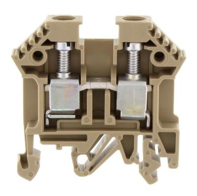
Feed-through terminal, Screw connection, Mounting type:Mounting rail TS 35/7.5 and TS 32, Rated cross-section: 10 mm², Width: 8 mm, Colour: Beige
