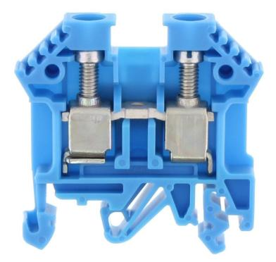
Feed-through terminal, Screw connection, Mounting type:Mounting rail TS 35/7.5 and TS 32, Rated cross-section: 10 mm<sup>2</sup>, Width: 8 mm, Colour: Blue
