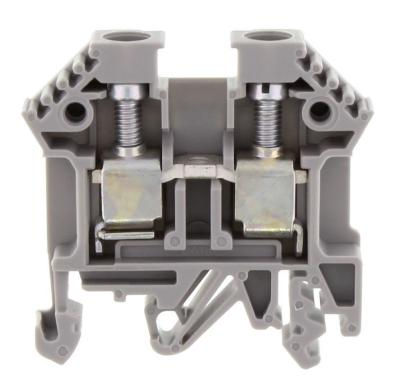
Feed-through terminal, Screw connection, Mounting type:Mounting rail TS 35/7.5 and TS 32, Rated cross-section: 10 mm², Width: 8 mm, Colour: Grey
