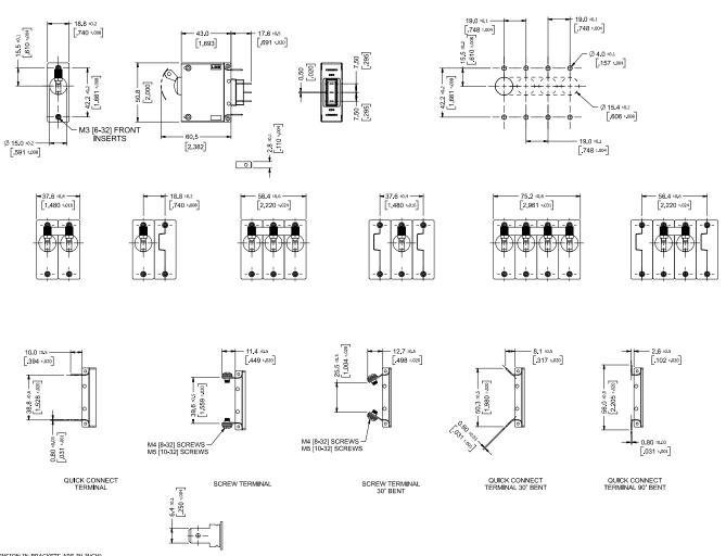
(DIMENSION IN BRACKETS ARE IN INCH) TOLERANCE ±0.4 UNLESS OTHERWISE SPECIFIED
