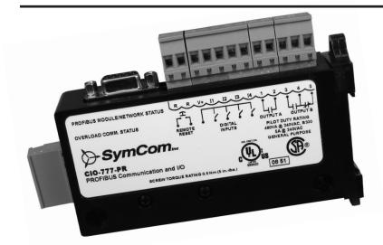
The CIO-PR module is a convenient, cost-effective Profibus interface device capable of providing discrete control and monitoring of motor starters, drives and other devices over a Profibus network.
