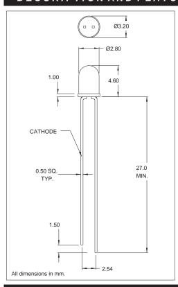
These T-1 LED lamps provide superior brightness compared to conventional LED lamps through the use of GaAlAs and improved GaP technologies. Intensities as high as 400 millicandela can be achieved with these lamps making them excellent choices for indicators in high ambient lighting conditions as well as for backlighting.
