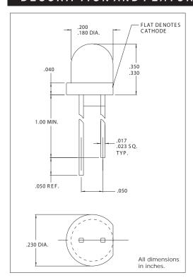
This T-1 3/4 HLMP4700 Series is a pin for pin replacement for Hewlett Packard lamps. All devices feature medium wide view angles. The design of the LED chips is optimized for low current applications and is far superior in luminous intensity compared to standard LED lamps at very low operating currents. These LED lamps are primarily intended for direct viewing. These lamps feature 4mW power and 2mA drive for low power TTL and CMOS circuits.
