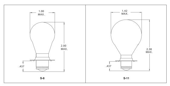
These unique Chicago Miniature Lamps are purpose built for the Marine Industry providing reliable performance in a wide variety of marine beacons. These lamps are manufactured in accordance with the United States Coast Guard, Ocean Engineering specification G-EOE-243B. Filaments and filament supports are specifically designed to meet these rigid specifications.
