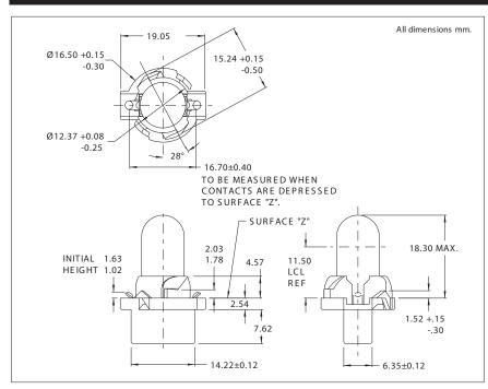
Mounting: Printed circuit board, twist-in
