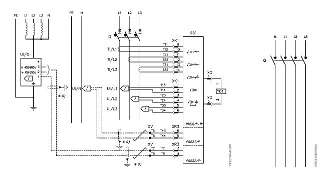
Three-pole circuit breaker with PR232/P-T8, PR331/P or PR332/P electronic trip unit
