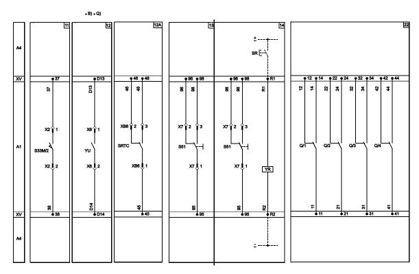
Auxiliary circuits for trip units
