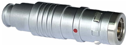
MMI-M0PGXXSXXB-IP67 IP67 Male Cable Plug, Straight Bend Relief, Size 0, Solder Cup
