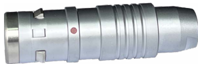
MMI-M1PGXXSXX-IP67 IP67 Male Cable Plug, Straight Back Nut, Size 1, Solder Cup
