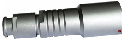
MMI-M0FGXXSXXB-IP67 IP67 Female Cable Plug, Straight Bend Relief, Size 0, Solder Cup
