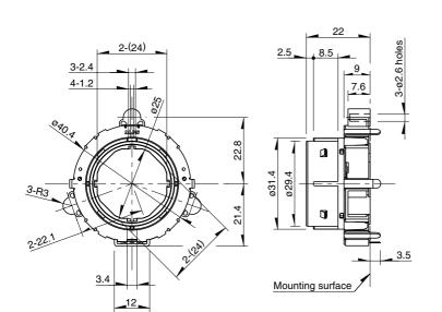
PC-board mounting hole dimensions (viewed from switch mounting face )
