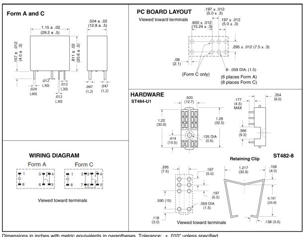
Dimensions in inches with metric equivalents in parentheses. Tolerance: ± .010" unless specified. \*ST482-8 - Contact Zettler for ordering details.
