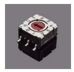
APEM's P36 Series DIP Coded Rotaries are available in SMT and through-hole configurations and are process sealed to ensure reliable operation. These dynamic switches are available in 10 and 16 positions in four output code configurations: BCD, BCD complement, hexadecimal and hexadecimal complement.
