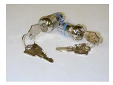
APEM's JD Series of Keylock Switches has a maximum current rating with resistive load of 4 amps at 125 VAC or 2 AMPS at 250 VAC. Expected life is 6,000 cycles at full load. Other electrical specifications include an initial contact resistance of 20 milliohms and maximum and dielectric strength of 1,000 V rms minimum at sea level.
