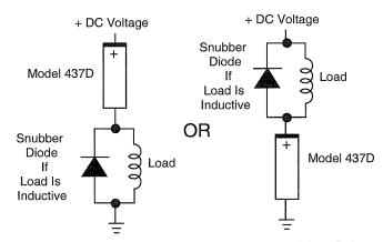
As a minimum protection against damage to the model 437D due to excessive transients generated by the inductive load circuit, always connect a snubber diode, or transient protector, across the load.
