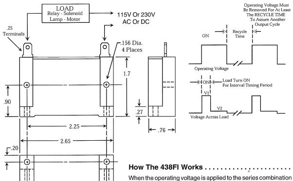
When the operating voltage is applied to the series combination of the 438FI and the load circuit, the 438FI turns ON, and the
