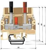
Disconnect test terminal block that allows longitudinal and transversal disconnection. Configuration provided with test plug socket upstream and a short circuit sleeve downstream the slide link (for short circuit plates type SCB/6/PO/2 or SCB/6/PO/4,
