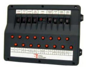
The heart of the ECS is the Electronic Control Processor (ECP). The ECP receives switching commands from the OCMs, translates the commands and activates or de-activates the appropriate circuits in the boat's electrical system. An ECP can control up to 16 separate circuits/accessories. Each circuit is protected by its own resettable thermal circuit protector.
