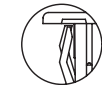
DETAIL VIEW VH1, VH3 & VH5 HOLE PLUGS (No wing serrations for ease of removal)
