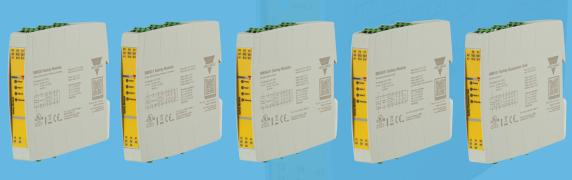
**SMS20** and **SMS31** safety modules are designed to provide for a safe interruption of safety circuits in applications with emergency stops, safety gates, safety magnetic switches, safety limit switches and electromechanical interlocks. They are also used to control safely the safety circuits of the lift car levelling, detection of uncontrolled movements of the cabin and the lift pit inspection, in compliance with the Lifts Standards EN81-20 and EN81-50.
