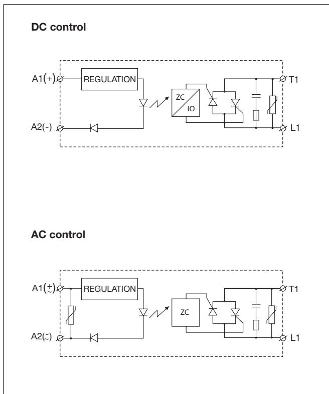
Note: Varistor on output is not included in the RGS1A69... models
