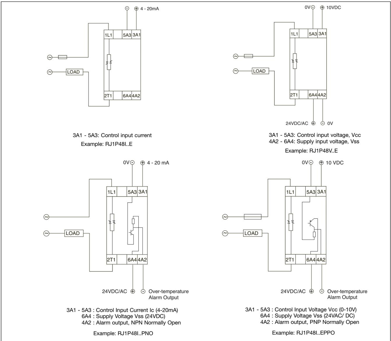
Note: For the RJ1P.V.E, it is possible to have the ground terminals of the supply and control power supplies used commoned. In the case, this common ground is connected either to terminal A2 or terminal A3. This is only applicable when a 24 VDC supply voltage is used. There should be no external direct link from Terminal A2 to Terminal A3.
