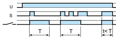
**(DE) Interval with control signal on.**
