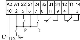
**BE:** Off-delay with control signal
