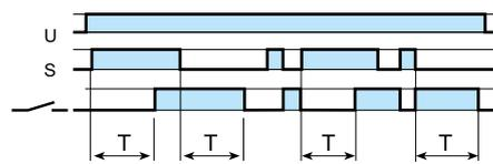
**(CEa) On- and off-delay with control signal.**
