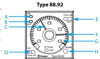
NOTE: time scales and functions must be set before energising the timer.
