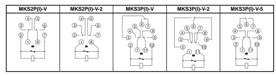
LED Indicator and Varistor Type (AC Coil)
