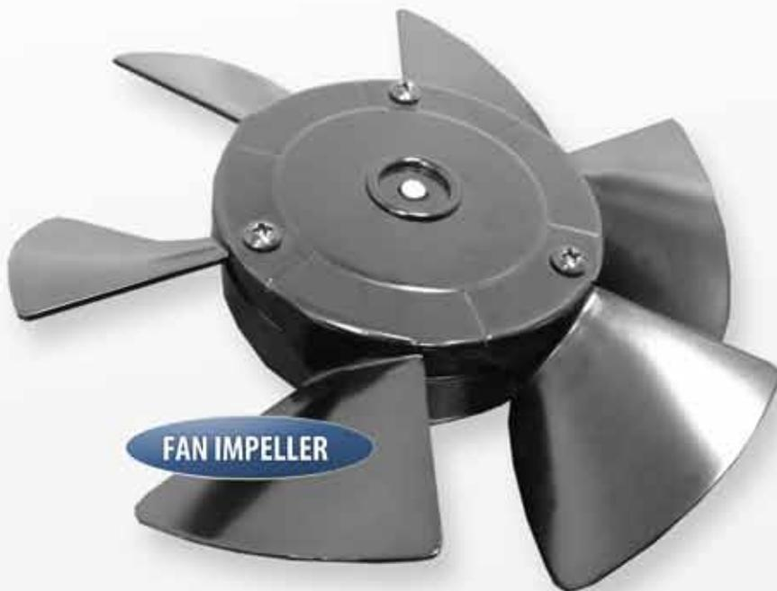
HPLC series axial fans feature a steel impeller and aluminum frame with a durable finish. The HPLC series impeller is a one piece forged part that allows better air flow performance, reduced noise, and long life in harsh environments. The frames have also been designed to reduce air resistance, manufacturing costs, and vibration. Plastic Impellers are available if the customer requires a higher static pressure and air quantity.
