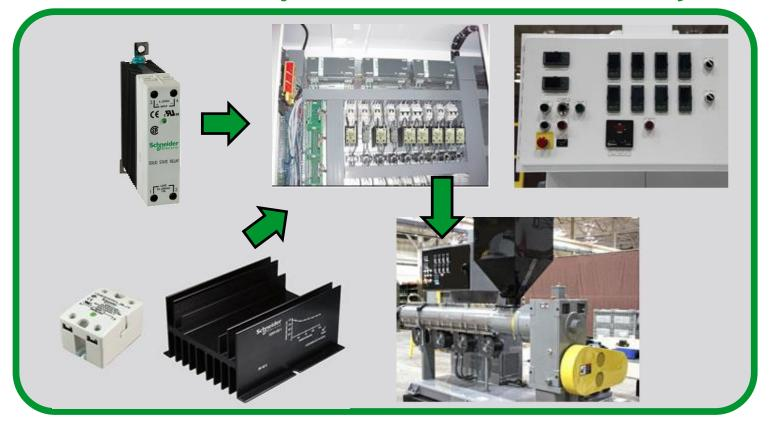
The Legacy SSRDIN and Class 6 Solid State Relays are an ideal combination of DIN rail and panel mount solid state relays for industrial plastic injection and extrusion equipment. DIN mount SSRDIN relays can switch up to 65A, and come with built-in heat sinks for quick installation. Class 6 relays can switch up to 125A with a number of available heat sinks for optimum thermal management. Both relays easily interface between the equipment's PLCs & ATVs and the load heating elements.
