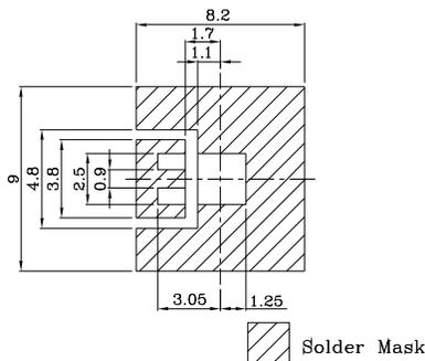
❖ The device has a single mounting surface. The device must be mounted according to the specifications.
