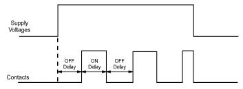
When the supply voltage is applied, the OFF cycle begins timing. Upon completion of the delay, the internal relay energizes and the ON cycle begins timing. The timer will continue cycling until the supply voltage is removed. ON and OFF cycles can be of equal or unequal durations.
