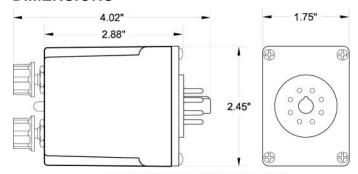
(dimensions have a tolerance of ± 0.06) Shows No Power Applied
